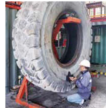
Earthmover tyre repair works at Timika, Indonesia
